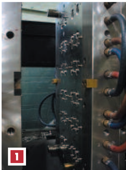
State-of-the-art equipment ensures high-speed, high-performing closure production. Clockwise: 1. Engel 300 ton Tiebarless injection molder features stainless steel molds. 2. High-speed vision inspection ensures closure quality. 3. Automated assembly systems prepare closures for customer delivery.
