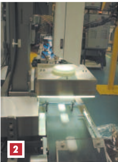
State-of-the-art equipment ensures high-speed, high-performing closure production. Clockwise: 1. Engel 300 ton Tiebarless injection molder features stainless steel molds. 2. High-speed vision inspection ensures closure quality. 3. Automated assembly systems prepare closures for customer delivery.
